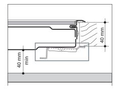
Fig. 5 Clamp adjustments depending on bench thickness
